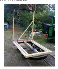
The new brake van with its basic frame. It is seen on gauging trials to ensure it didn't scrape the greenhouses or wagon shed.
