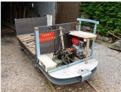
Introducing you to the Terry Stanhope motorised truck which has had a new engine and brakes fitted and its timbers treated with preservative
